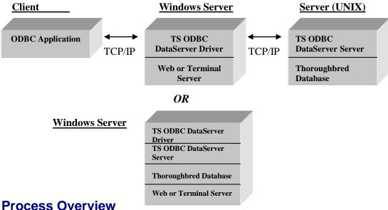
The process to get your Thoroughbred data to appear in an ODBC-enabled application starts with a successful installation of the TS ODBC DataServer components. Once completed, the TS ODBC DataServer Expose Utility is executed to create the Data Source entries from Thoroughbred data definitions. For Single-Tier installations the expose process is executed on the workstation system. For Multiple-Tier installations it is executed on the server system.
