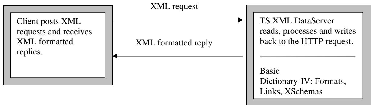
The TS XML DataServer also supports XML requests from within a TS Environment by CALLing the TS XML Request Manager. The TS XML Request Manager accepts standard Thoroughbred selection parameters, constructs a properly URL encoded HTTP query string and manages all communication with the server process running on the remote server.
